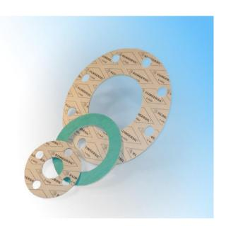
Optimised combination of synthetic fibres and glass-fibre bound with NBR. Premium quality jointing with high temperature resistance in steam and water as well as excellent resistance to oils and hydrocarbons.
